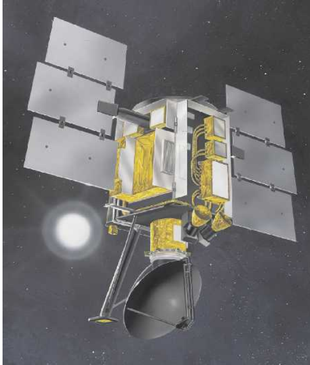
FIG. 2. The SeaWinds instrument on board QuikSCAT. The rotating disk antenna is 1 m in diameter (courtesy NASA/JPL).
